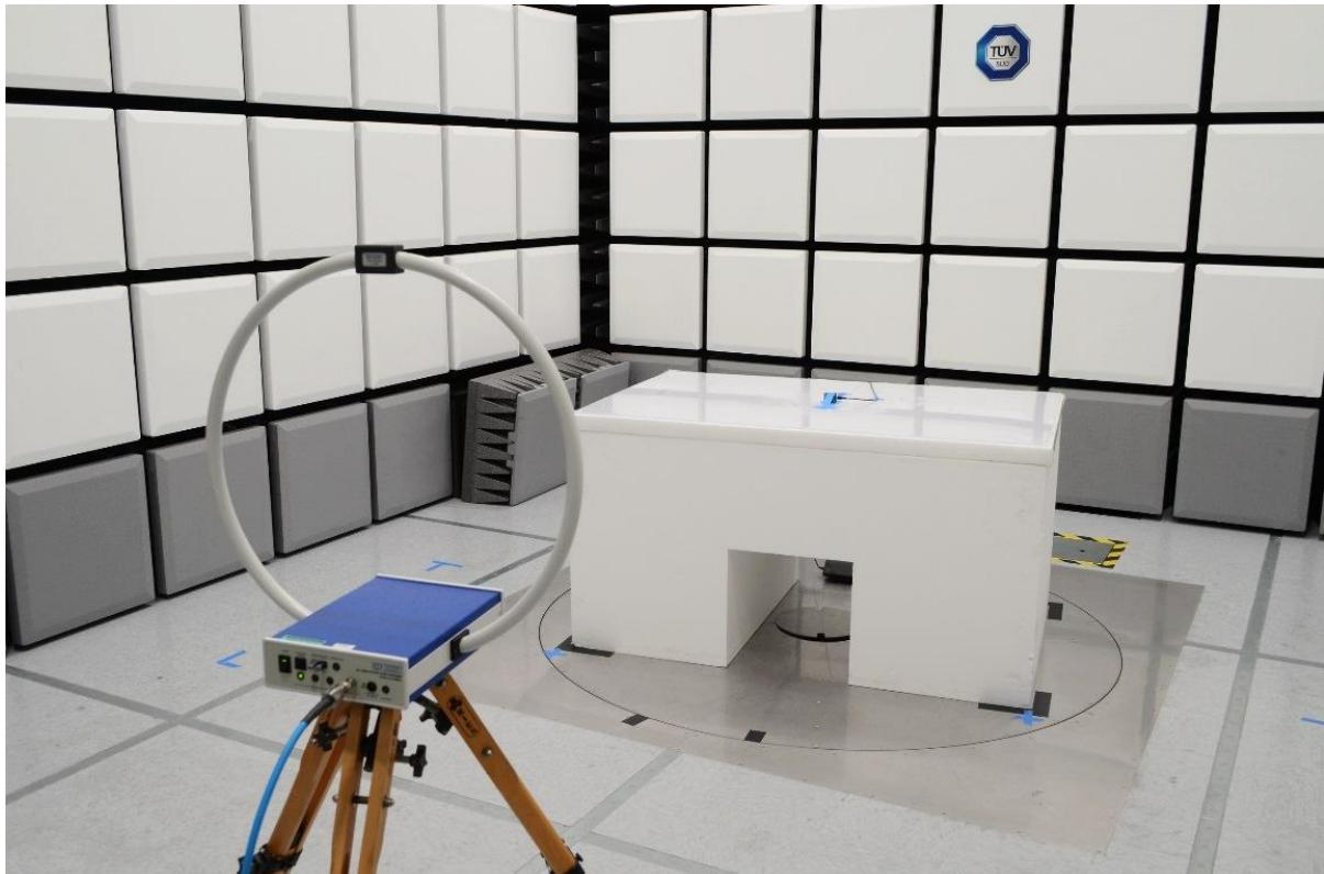
**Radiated Emissions Test Setup (9 kHz to 30 MHz Front)**
