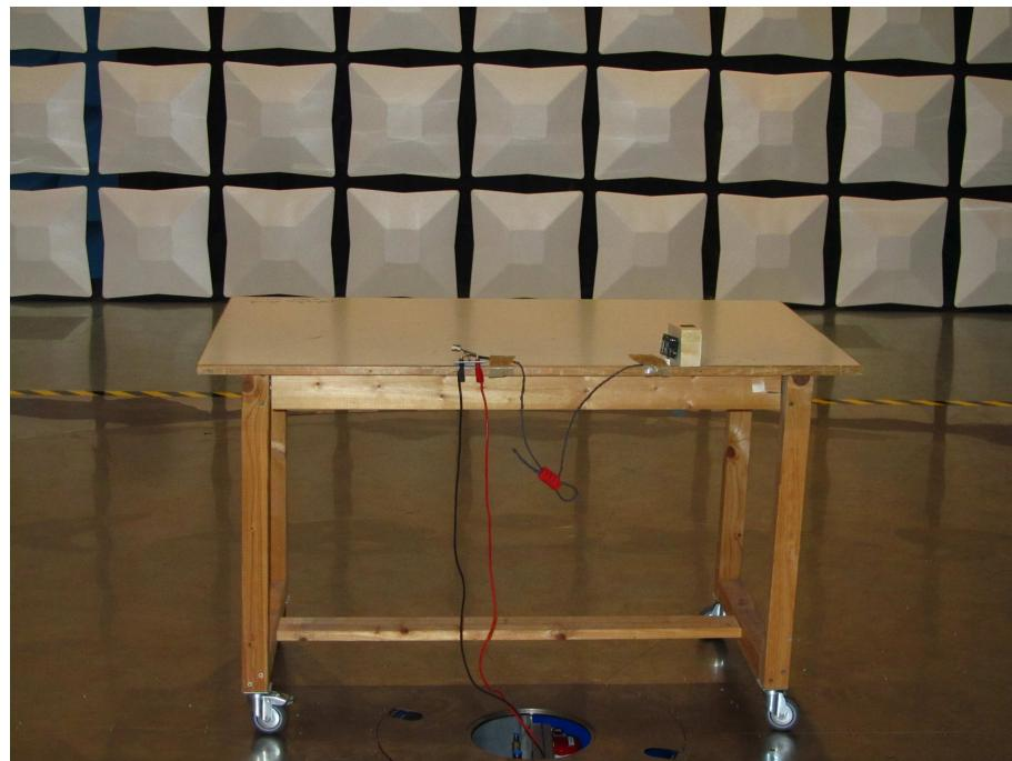
**Test setup for radiated emission measurement
