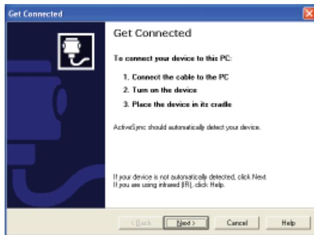
4. ActiveSync installation is finished. Please turn on and put the STM-8800 unit on to the cradle with USB cable connected to the PC. (use USB 2.0 or higher)
