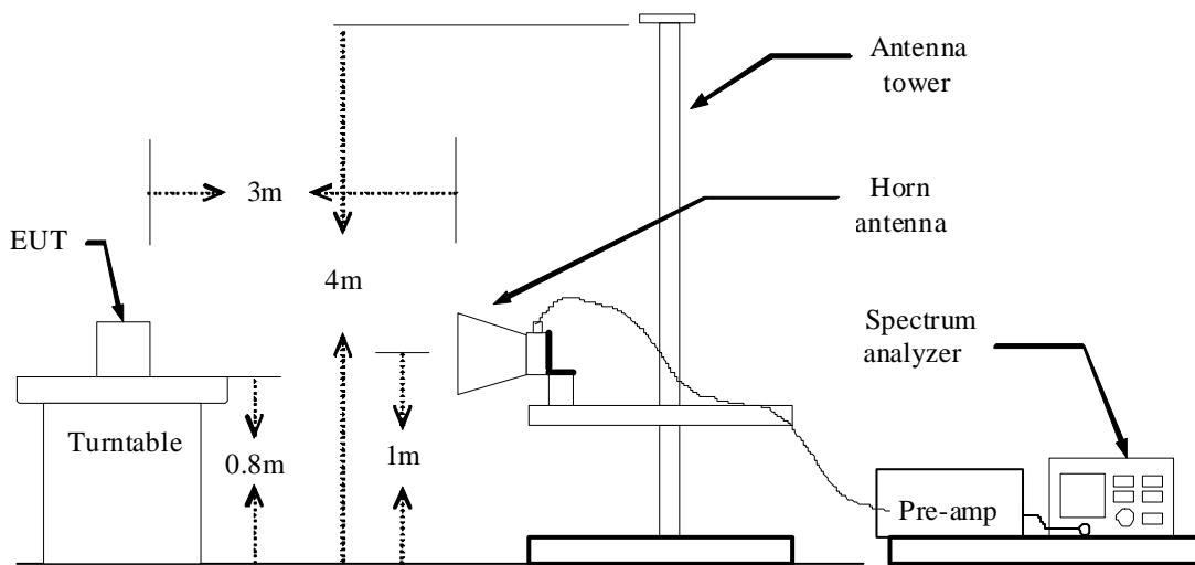
The radiated emission tests were performed in the 3 meters chamber 966 test site, using the setup accordance with the ANSI C63.4-2003. The specification used was the FCC 15.209, and FCC 15.247 limits.
