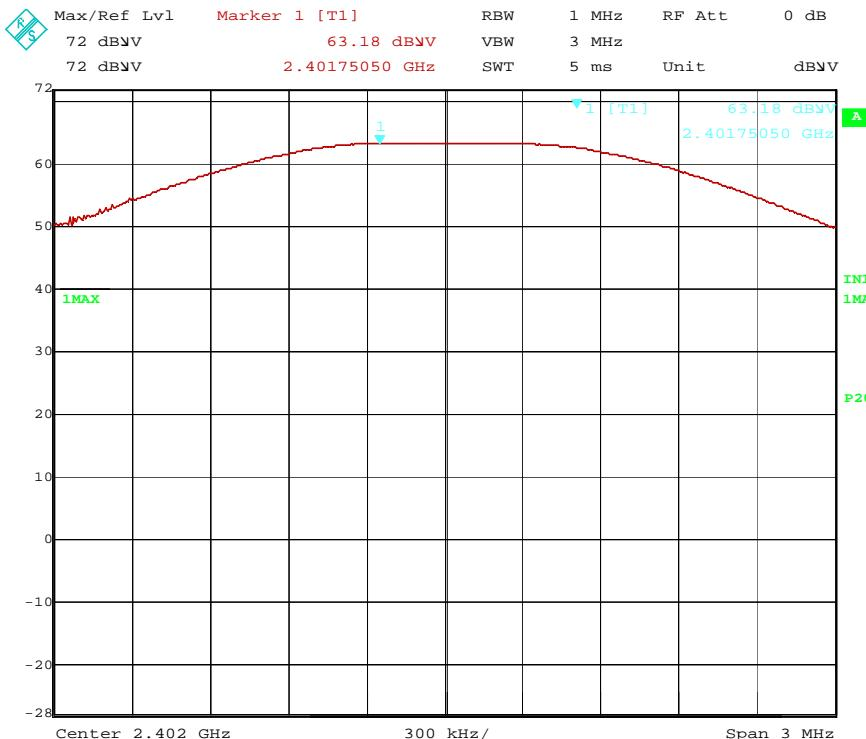
The highest antenna gain is 0 dBi. Therefore no reduction of the Peak power limit is necessary and the EIRP is the same as the conducted power.
