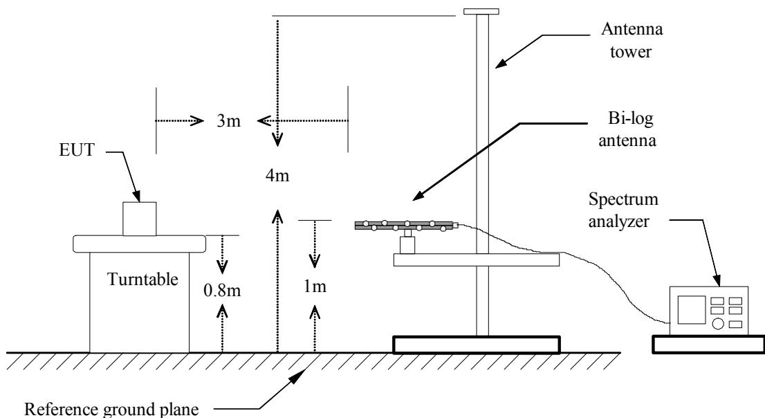
**Above 1 GHz**
