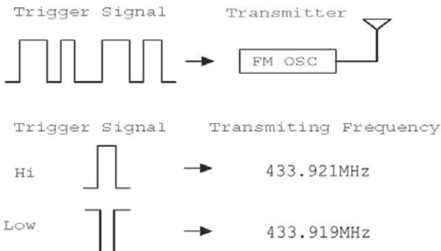
This EUT works as a FM modulation. Signal HI will trigger FM OSC to generate a 433.921MHz frequency and signal LOW will trigger FM OSC to generate a 433.919MHz frequency. It is only 0.002MHz deviation, so that there is no duty cycle on it.
