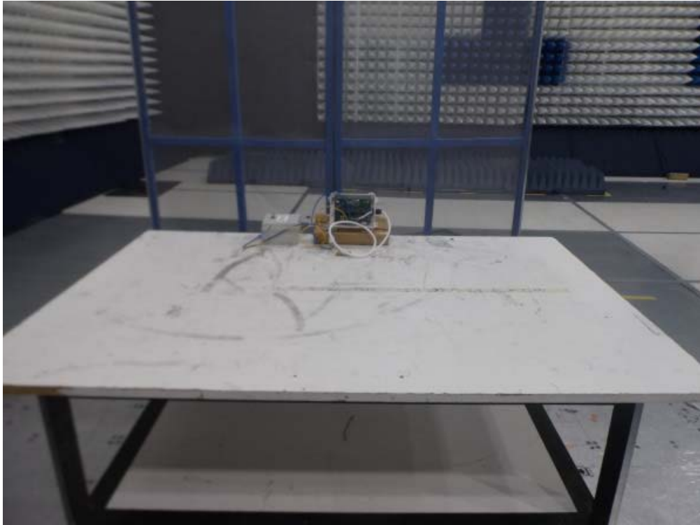
AC Powerline Conducted Emissions, front view
