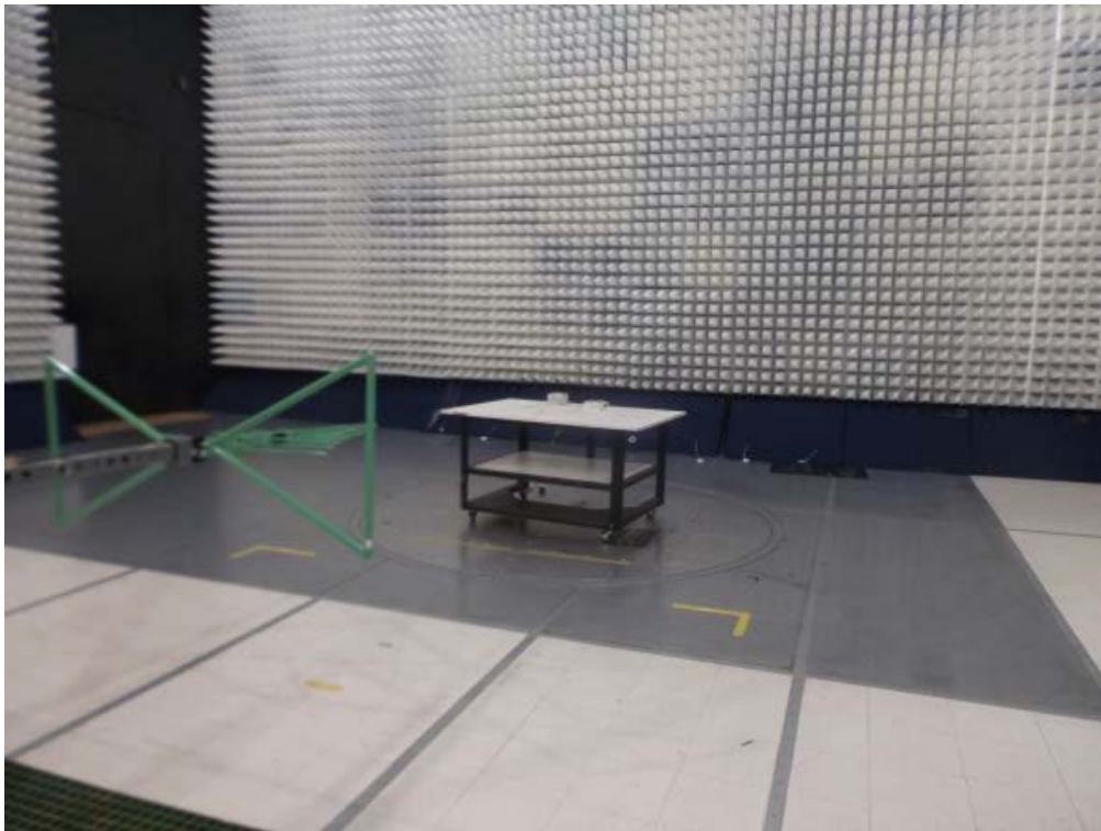
Radiated Emissions below 1 GHz, rear view
