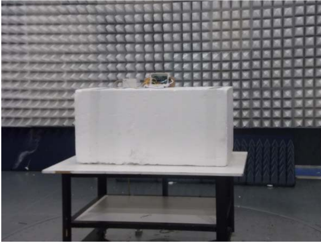
Radiated Emissions above 1 GHz, front view
