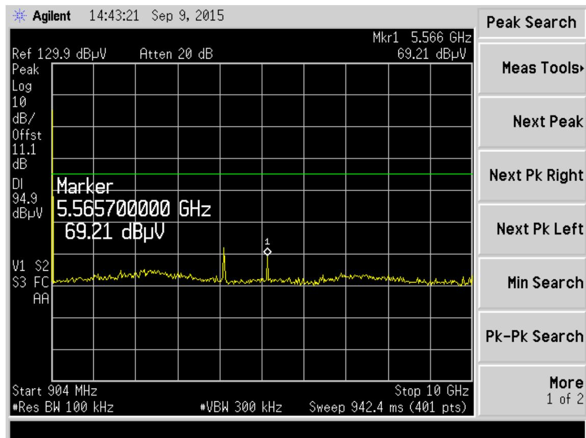
The display line is the limit line of 20 dB below the carrier.
