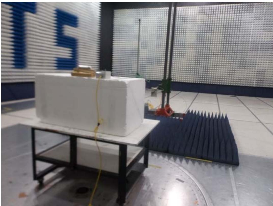
**8.5 Test/Data:****Client:** TPI Corporation**Model Number:** RFR-5**Project Number:** G100315802**Tested By:** MTS**Date:** 09/02/2015**Frequency Range (MHz):** 30 to 1000**Input power:** 24 Vac**Receiver:** R&S ESU40**Antenna:** Chase 2622**Cables:** TT-7+MP3+E-207**Preamp:****Test Distance (m):** 3**Limit:** FCC15 Class B-3m
