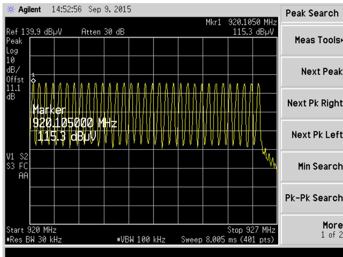
Number of Hopping Channels Measured = 64 channels
