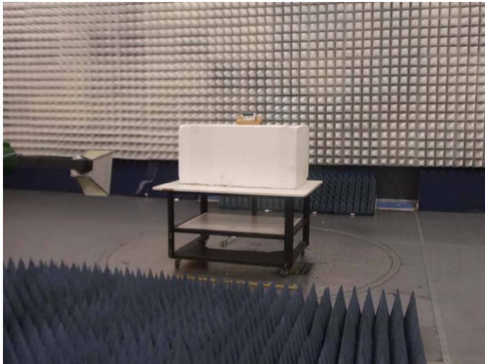
**7.5 Test Data:****Client:** TPI Corporation**Model Number:** RFT-1**Project Number:** G100315802**Tested By:** MTS**Date:** 10/16/2015**Frequency Range (MHz):** 30 to 1000**Input power:** 3 Vdc, 2 x AAA batteries**Receiver:** R&S ESU40**Antenna:** Chase 2622**Cables:** TT-7+TW2+E-207+E-209**Preamp:** PAM-0202**Test Distance (m):** 10**Limit:** FCC15 Class B-10m
