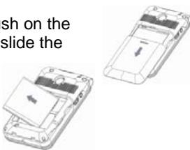
**3.** Remove the battery by lifting from the Left edge.
