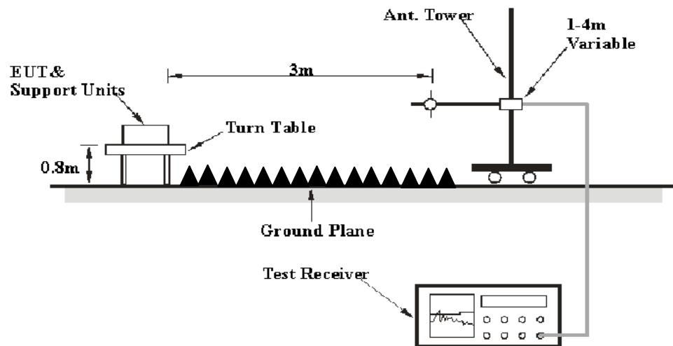
The radiated emission tests were performed in the 3 meters chamber test site, using the setup accordance with the ANSI C63.4 - 2009. The specification used was the FCC §15.209 and §15.231.
