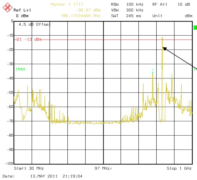
Fundamental test with Band Reject Filter
