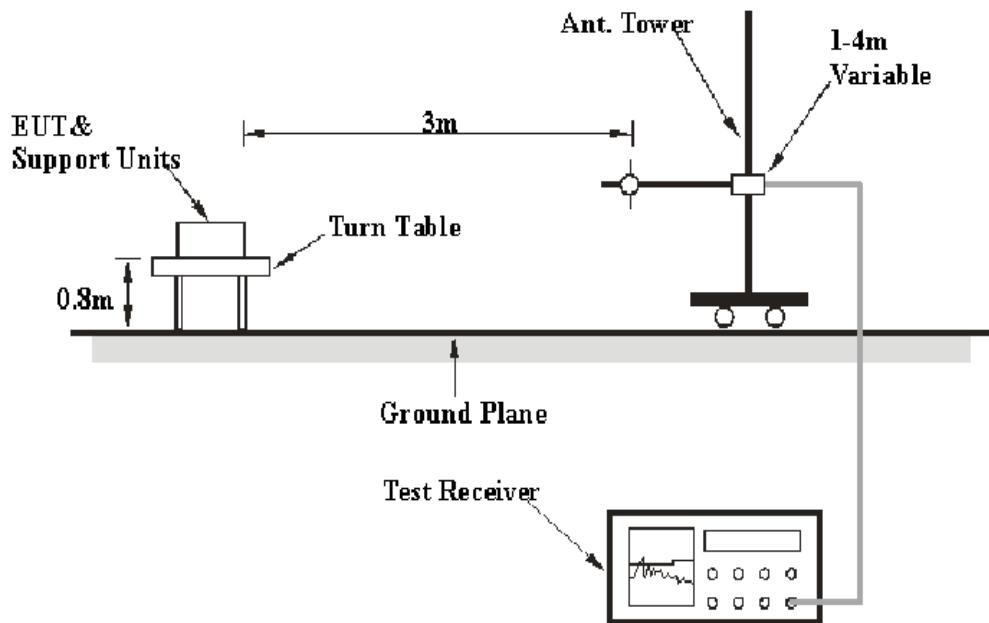
The radiated emission tests were performed in the 3 meters chamber test site, using the setup accordance with the ANSI C63.4 - 2009. The specification used was the FCC §15.209 and §15.231.
