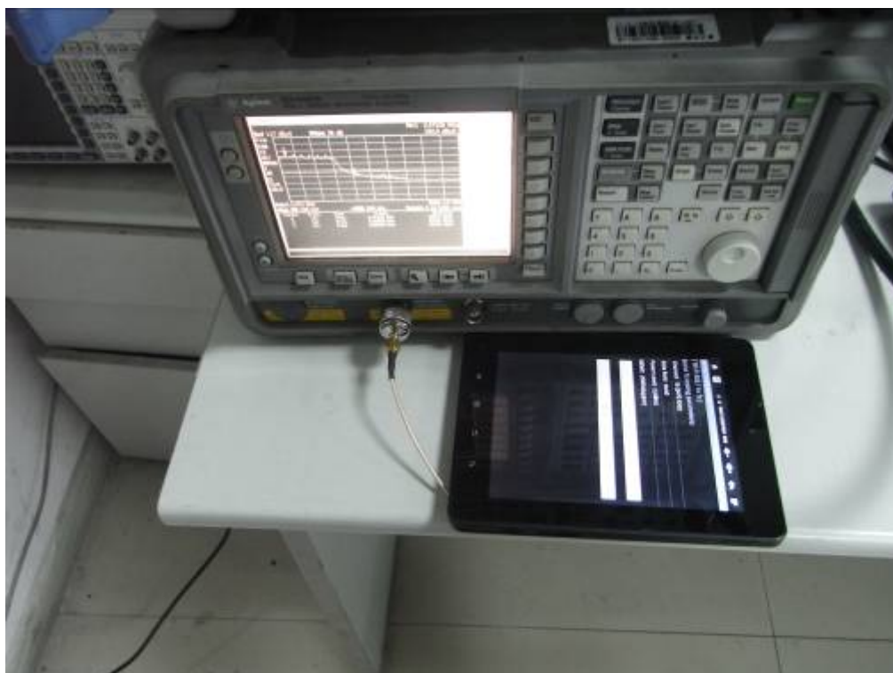
CONDUCTED SPURIOUS EMISSION TEST SETUP
