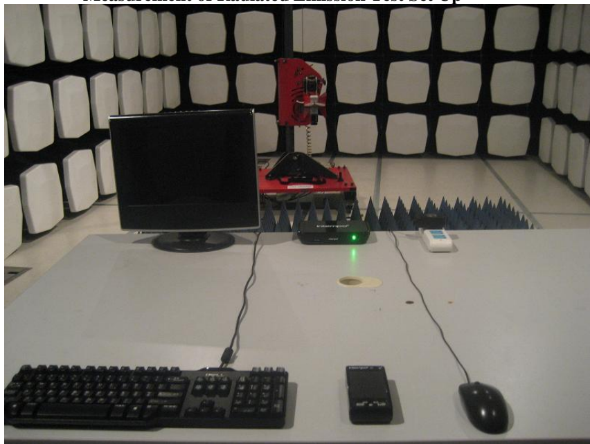
Measurement of Radiated Emission Test Set Up
