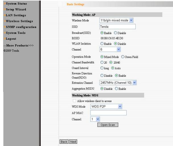
Bridge (WDS) working mode includes: Point to Point Bridge (WDS P2P), Point to Multipoint Bridge (WDS P2MP), Wireless Repeater (Repeater). Users can select the mode according to need. Please refer to Chapter 4.1.2 for detailed introduction.
