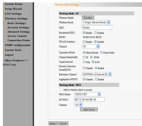
This page includes the AP and WDS parameter setting. AP parameter setting can change SSID and enable/ disable wireless feature.
