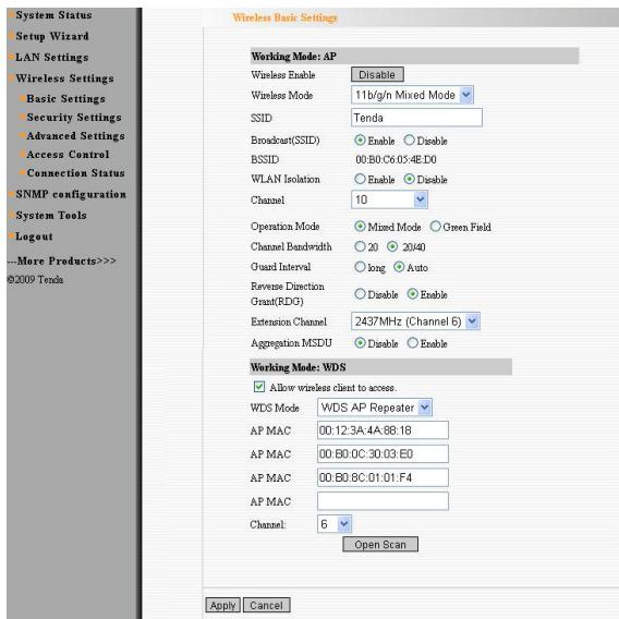
When the users select “permit wireless client to access”, AP can also be used as “Wireless Access Point” to allow the access of wireless client when it is used as a wireless bridge. The basic settings of wireless repeater are divided into two parts: one part is the basic setting in AP mode (See 4.1.1.2); another part is the basic setting in WDS mode (See 4.1.2.2).
