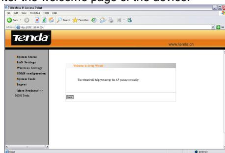
You can select “Running Status”, “LAN Settings”, “Wireless Settings”, “SNMP Settings” and “System Tools” on the left menu. Click “Next” to enter the wireless working mode setup page. WAP123N supports two working modes: wireless AP (AP), Bridge (WDS). Select a working mode to configure the settings. For more details please refer to the following chapters.
