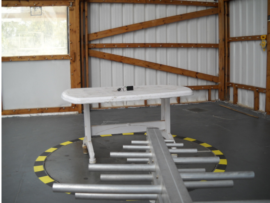
Photograph No.6 Setup for occupied bandwidth measurements
