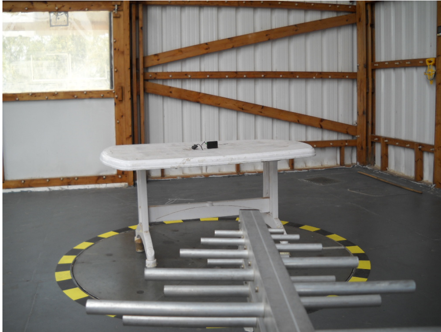
Photograph No.3 Setup for radiated emission measurements at OATS from 30 to 1000 MHz
