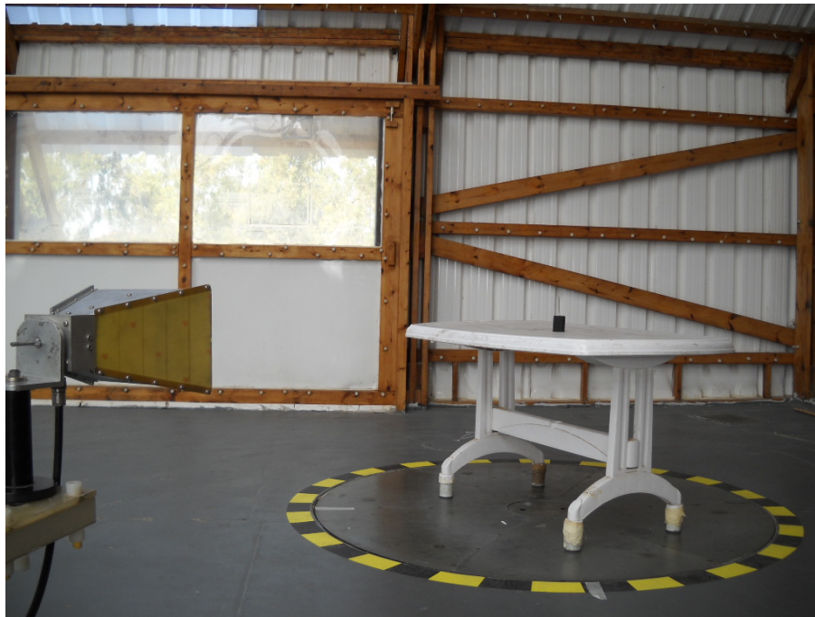
Photograph No.5 Setup for radiated emission measurements at OATS above 1 GHz
