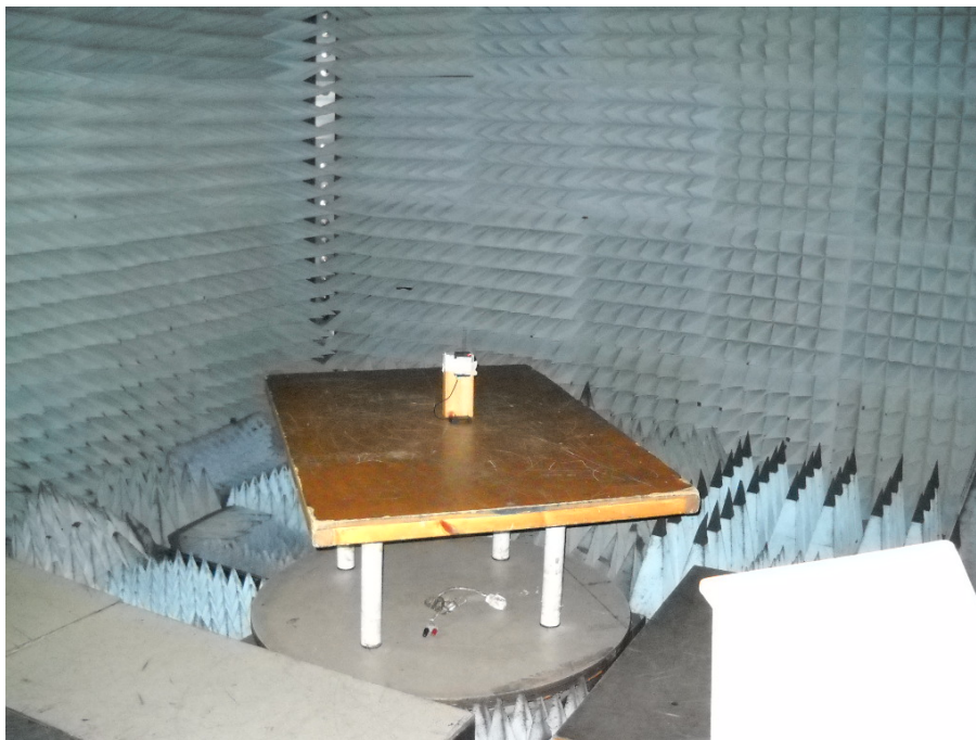
Photograph No.4 Setup for radiated emission measurements in the anechoic chamber above 1 GHz
