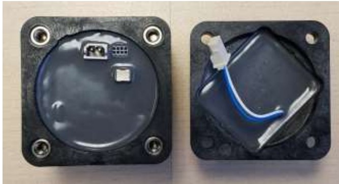
Figure 1: Install WASP™ Battery Board
