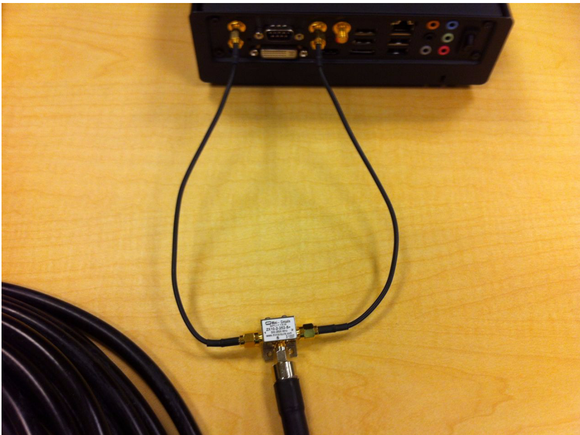
Hub detail showing connection to external splitter/combiner
