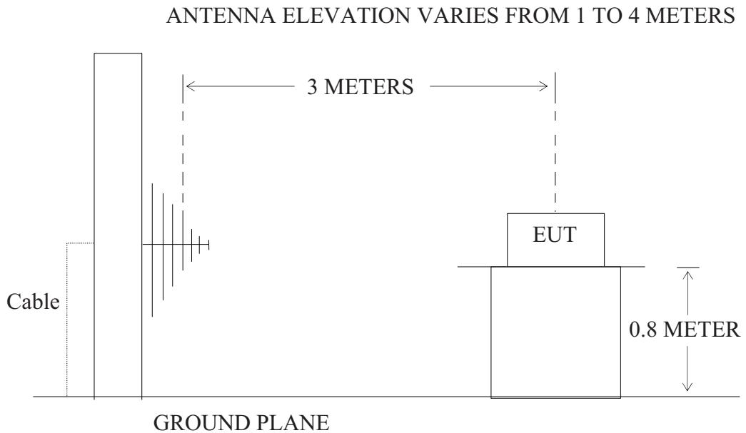
(EUT: FM Transmitter with Memory slot and USB)
