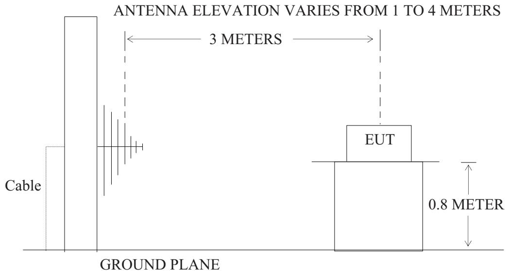
(EUT: FM Transmitter with Memory slot and USB)
