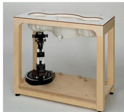
The ELI4 Phantom also is a fiberglass shell phantom with 2mm shell thickness. It has 30 liters filling volume, and with a dimension of 600mm for major ellipse axis, 400mm for minor axis. It is intended for compliance testing of handheld and body-mounted wireless devices in frequency range of 30 MHz to 6GHz. ELI4 is fully compatible with standard and all known tissue simulating liquids.
