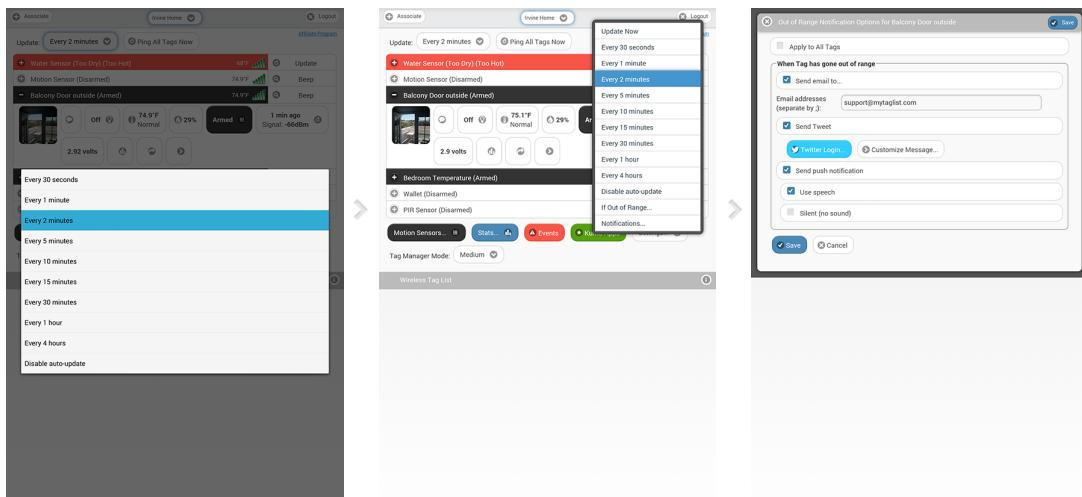
At the top of tag list screen, choose any of the Record: "Every ..." options. This is the data logging interval. The default is every 10 minute to balance battery life vs. amount of data logged and out-of-range notification delay.
