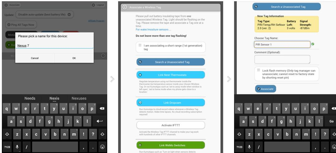
First time when the app is launched, it may ask for the name to use to identify current device to enable/disable push notification later. Click "OK" and click the "+ Associate" button at the upper left corner.
