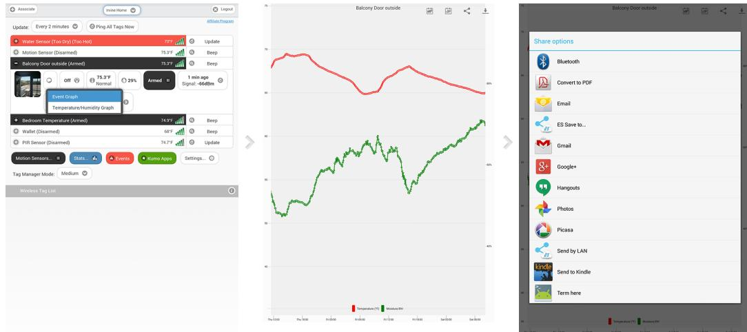
Temperature is logged periodically for each tag at the interval specified at **Step4, "Out-of-range Notification."** To view logged data, click the graph button and choose "Temperature Graph".
