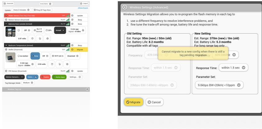
When a tag failed to be updated, its "Beep" button becomes a "Migrate Setting" button. Click on it to retry updating its flash memory. Before update succeeds, Tag Manager communicates with that Tag using the old wireless setting. Alternatively, click the ">" button and then "Use new wireless setting" if in fact the tag has migrated successfully but did not get recognized that way.
