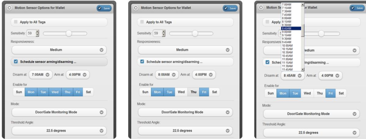
By setting an auto-arming/disarming schedule, you can specify time of day to disarm (for example, in the morning), and arm (for example, after dark), for each of the checked days of the week. To make motion sensor armed over the weekend, simply setting an "Arm at" time later than "Disarm at" time, and uncheck Saturday and Sunday.
