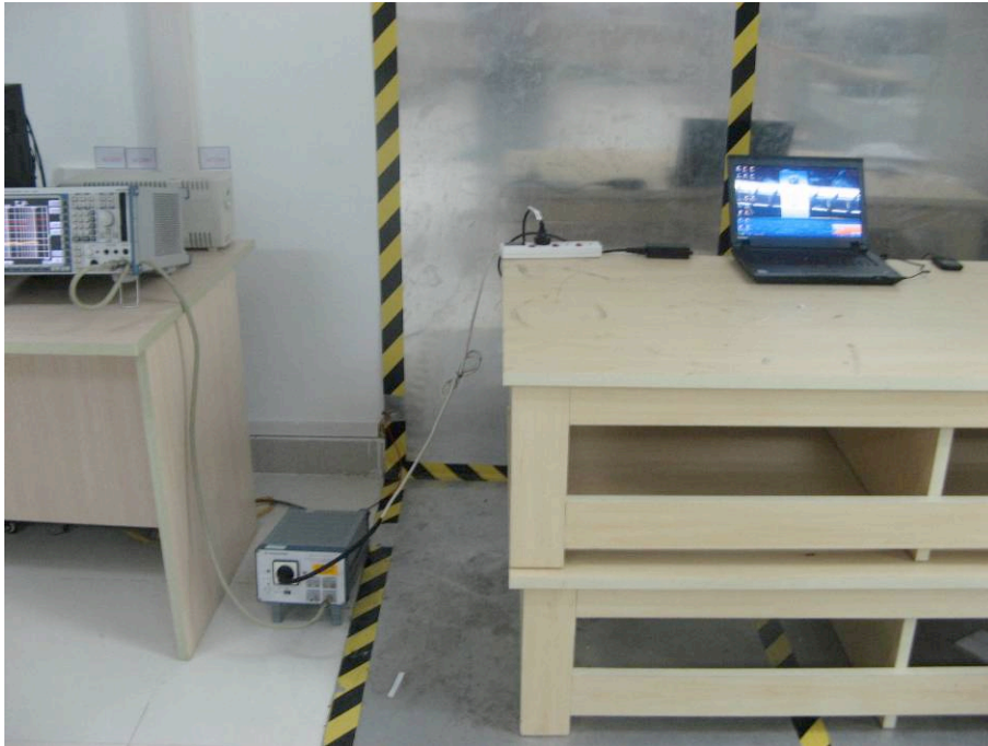
FCC LINE CONDUCTED EMISSION TEST SETUP
