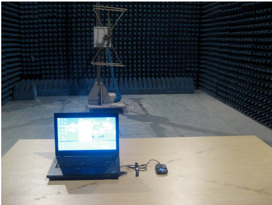
FCC RADIATED EMISSION TEST SETUP
