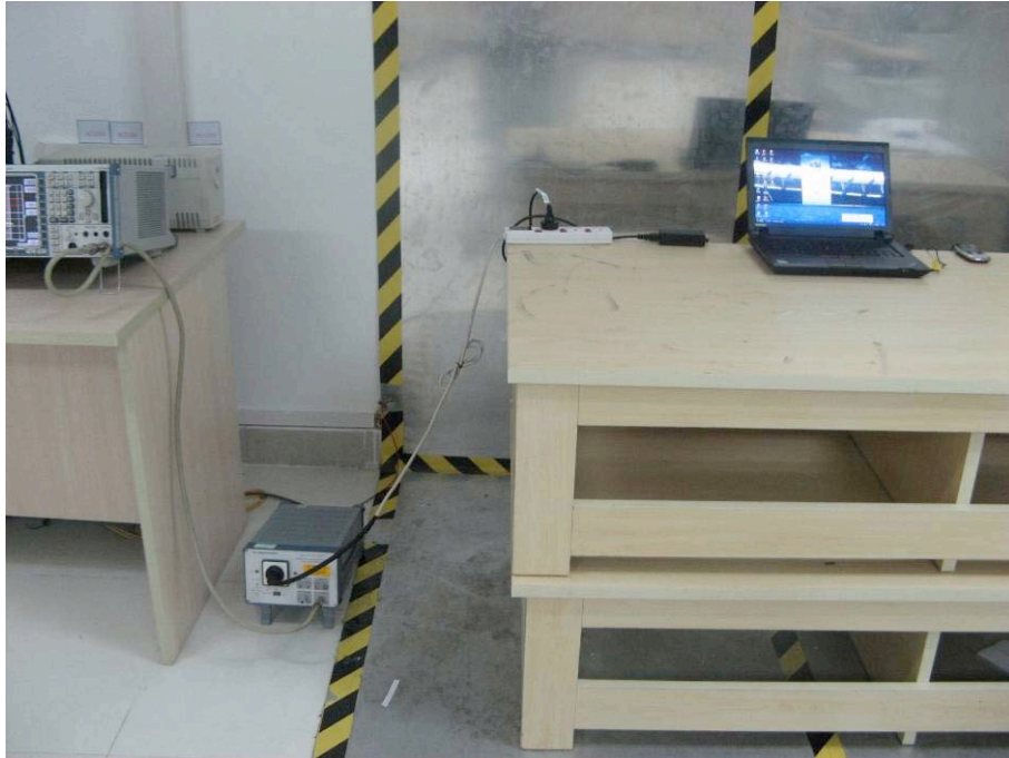
FCC LINE CONDUCTED EMISSION TEST SETUP
