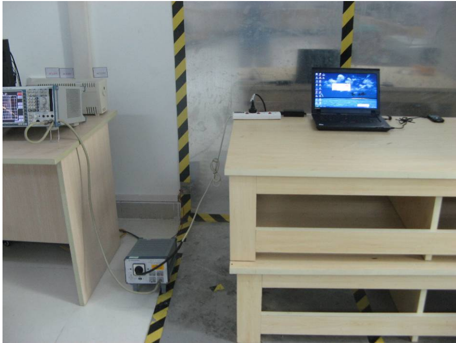
FCC LINE CONDUCTED EMISSION TEST SETUP
