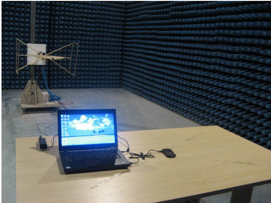
FCC RADIATED EMISSION TEST SETUP
