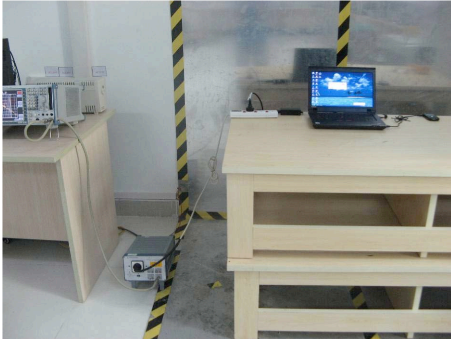
FCC LINE CONDUCTED EMISSION TEST SETUP
