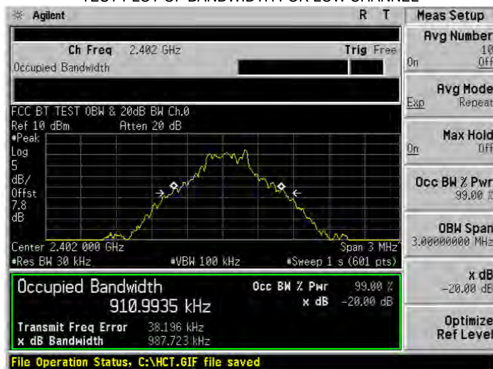
TEST PLOT OF BANDWIDTH FOR LOW CHANNEL
