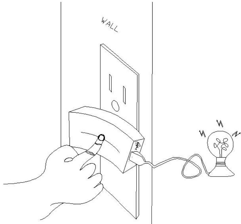
6. In the SWITCH mode, manually turn the connected lighting ON/OFF by pressing the button.
