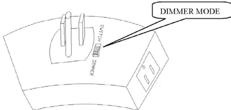
2. Plug the lamp into the Dimming Switch module outlet (C). Outlet (B) is always On and outlet (C) is Z-Wave control. Ensure that the loading does not exceed 330 Watts.
