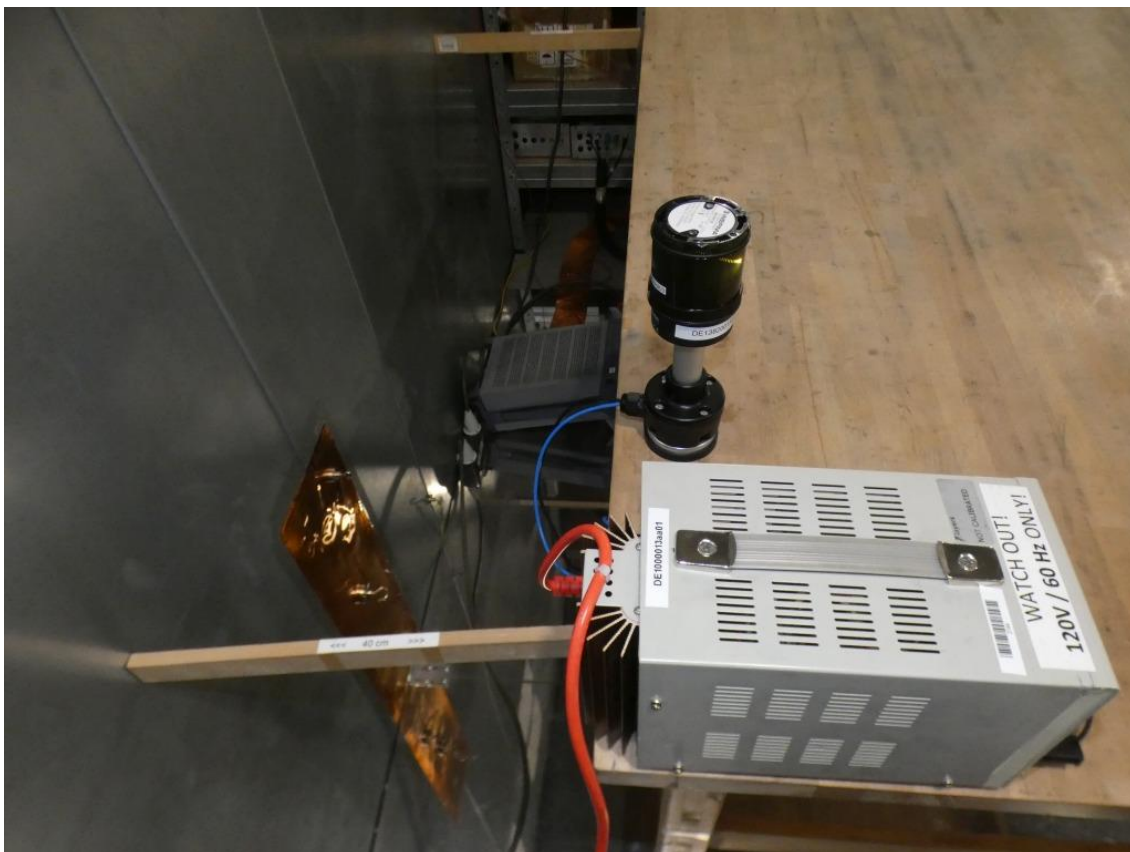
Photo 2: Setup for conducted emissions, top/left view
