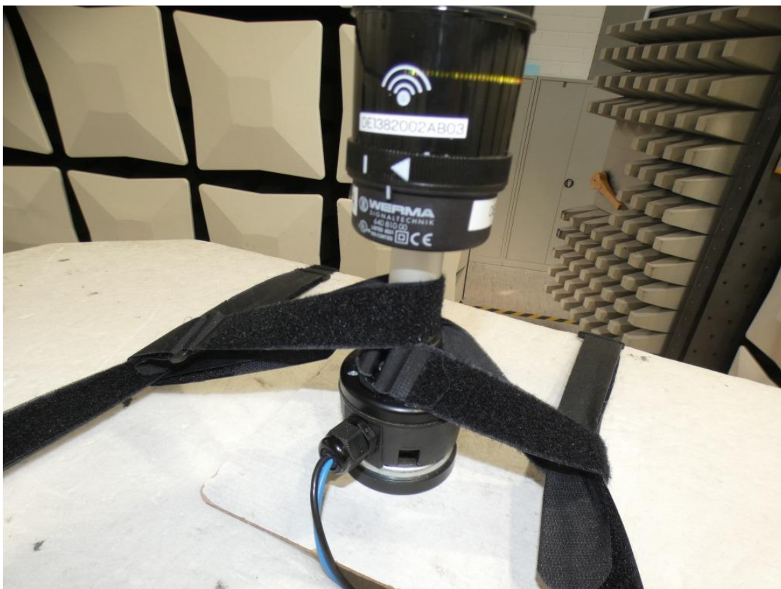
Photo 6: Setup for radiated emissions > 1 GHz, detail view
