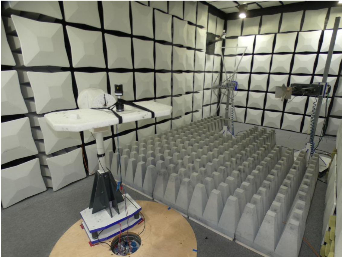
Photo 5: Setup for radiated emissions > 1 GHz, rear side view
