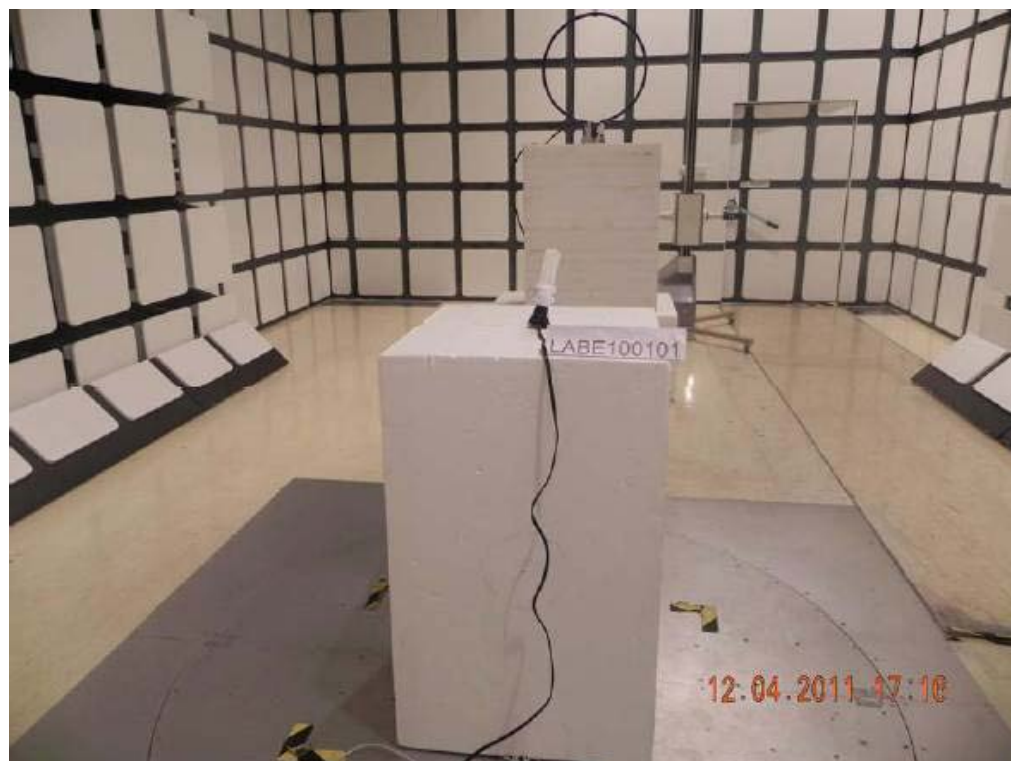
Back View of Radiated Emission (9 kHz-30MHz) Test Setup:
