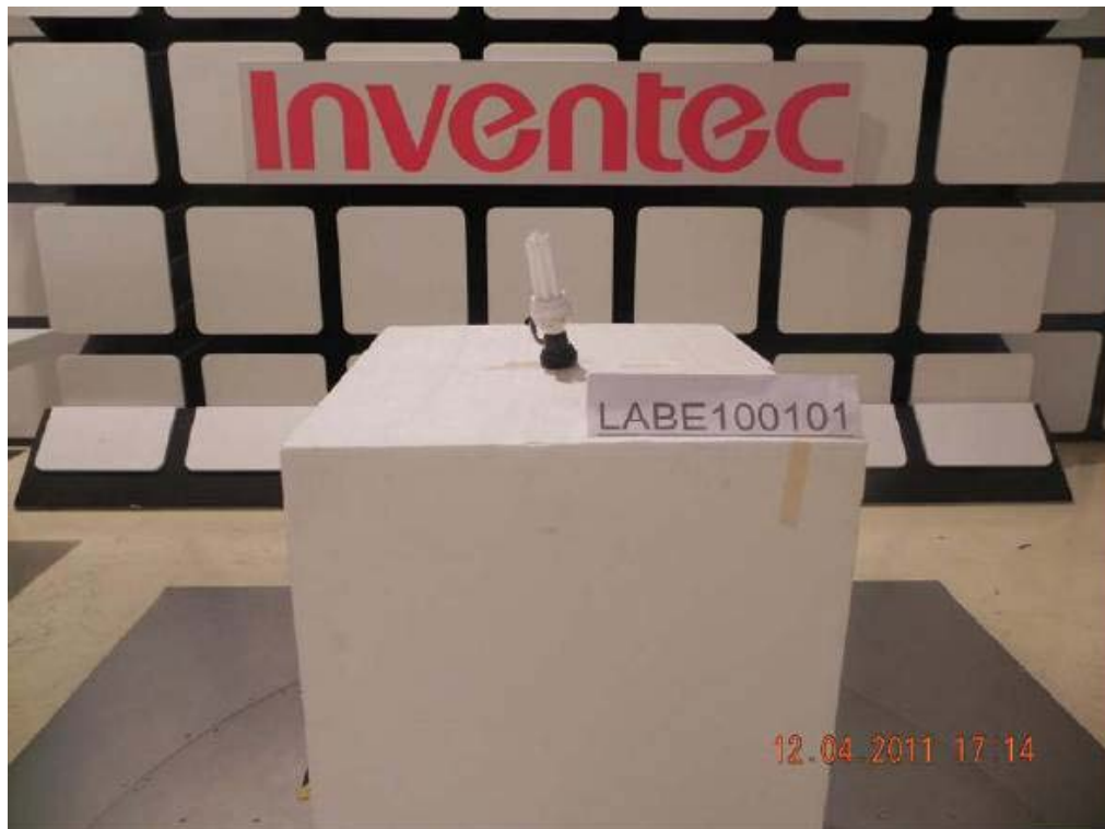
Front View of Radiated Emission (9 kHz-30MHz) Test Setup:
