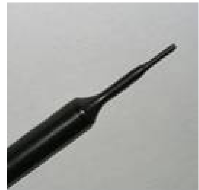
Figure 2. EX3DV4 E-field Probe
