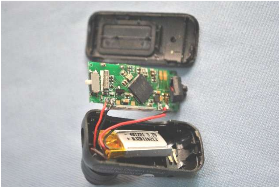
Main & RF board component side
