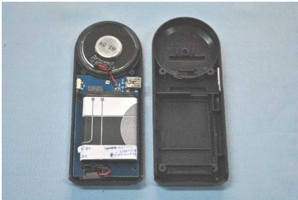
Main&RF board component side
