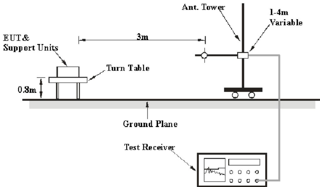
The deactivation test was performed in the 3 meters chamber test site, using the setup accordance with the ANSI C63.4 - 2003. The specification used was the FCC 15.231(a) limits.
