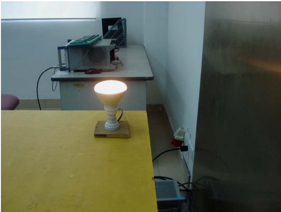
AC Line Conducted Emission Test Setup - Side View
