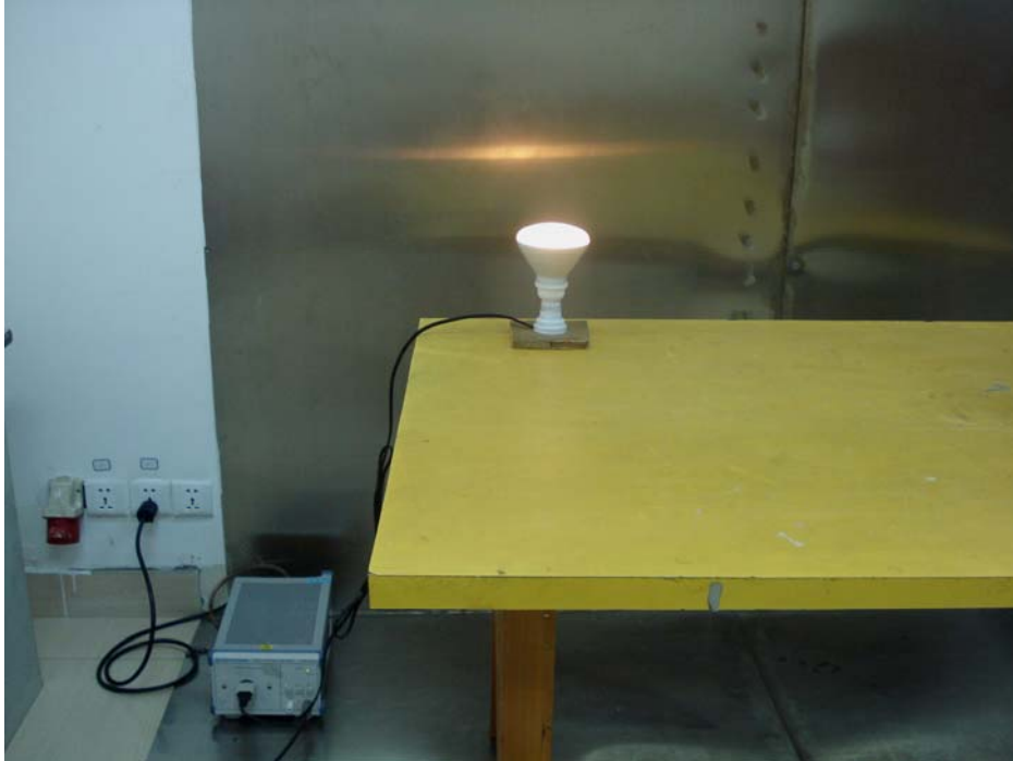
AC Line Conducted Emission Test Setup - Side View
