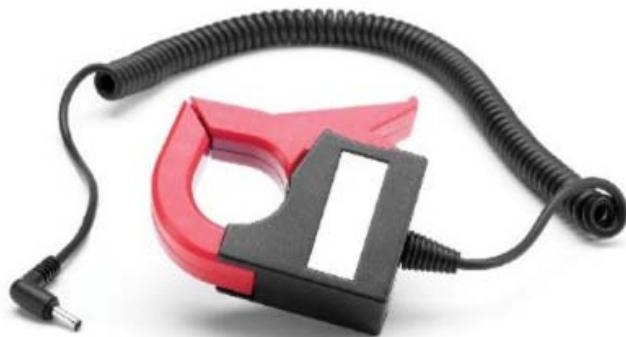
The Sensor Clamp immediately starts to sensor the current and the energy monitoring system starts to work. The LCD screen of the Display Unit should now display the electricity information of the monitored object in real time.
