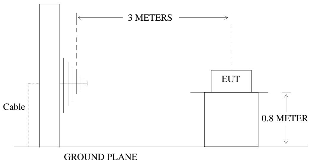
(EUT: Electricity Energy Monitoring System)
