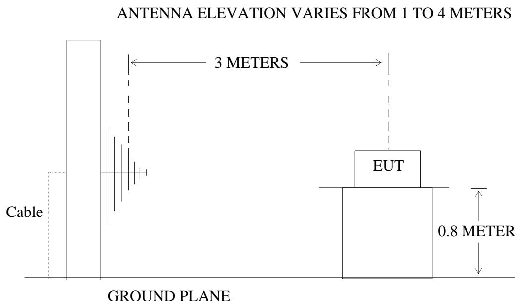
(EUT: Electricity Energy Monitoring System)
