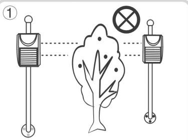
**Note 1:** Make sure that there is no obstacle between the transmitting terminal and the receiving terminal.
