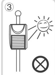
**Note 3:** Keep the infrared light hole exposed to direct sunlight.
