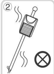
**Note 2:** Never install the detector at an inclined angle.
