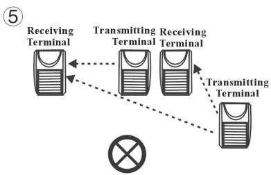
**Note 5:** Multiple detectors shall be installed for long-distance alarm in accordance with the installation instructions shown in the above-mentioned figure to avoid mutual interference among beams.
