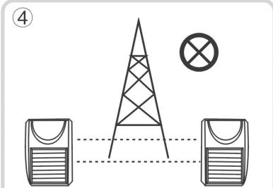
**Note 4:** The high-voltage tower and the signal tower may influence wireless transmission.
