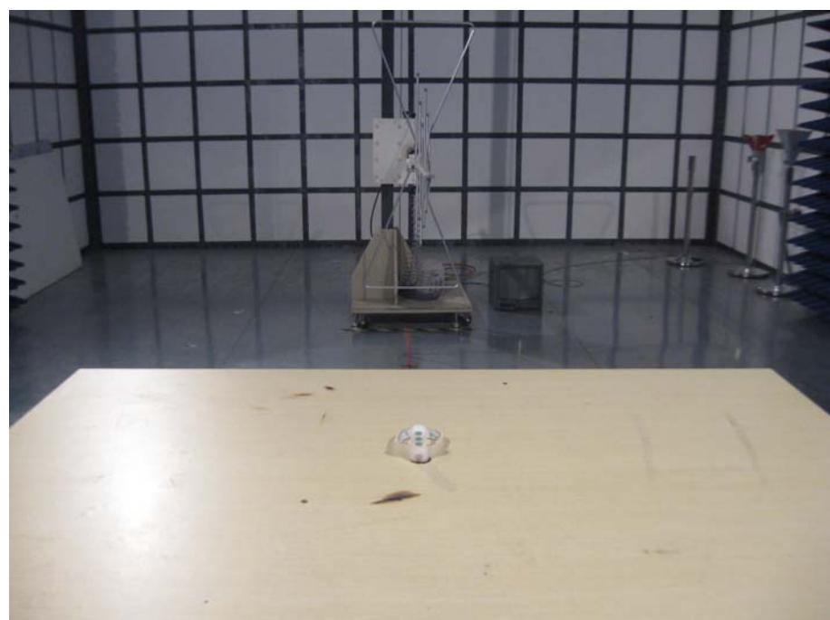
*Test Model: Charging*
