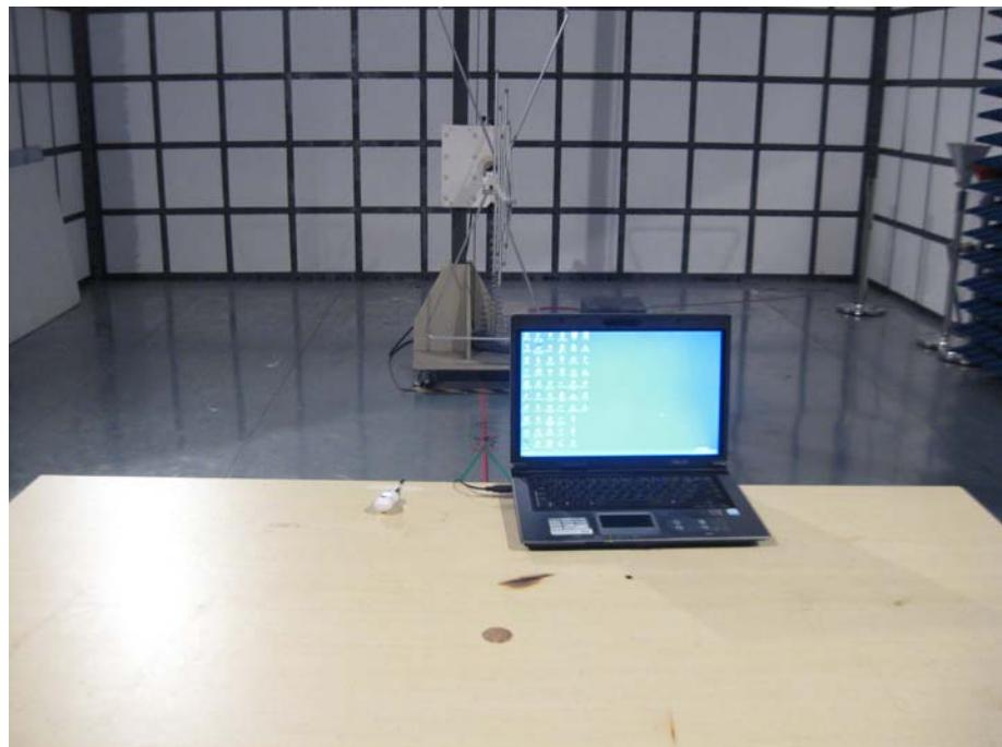
**Radiation Emission Test Setup (Above 1GHz)**
