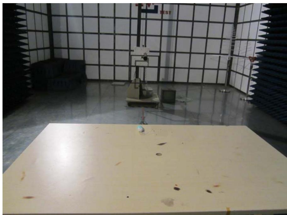
**Radiation Emission Test Setup (Above 30MHz)**
