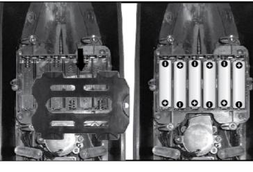
5) Replace the battery door and turn the battery door locks, make sure it is secure.
