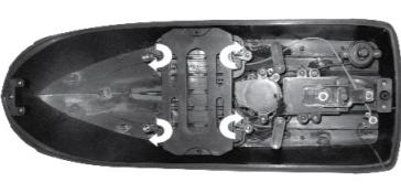
4) Remove battery door and insert 6 AA batteries (not included).
