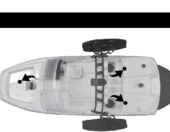
2) Open the top cover to reveal battery compartment.
