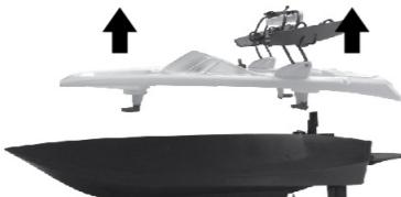
3) Open battery door by turning the four locks located on the battery doors.
