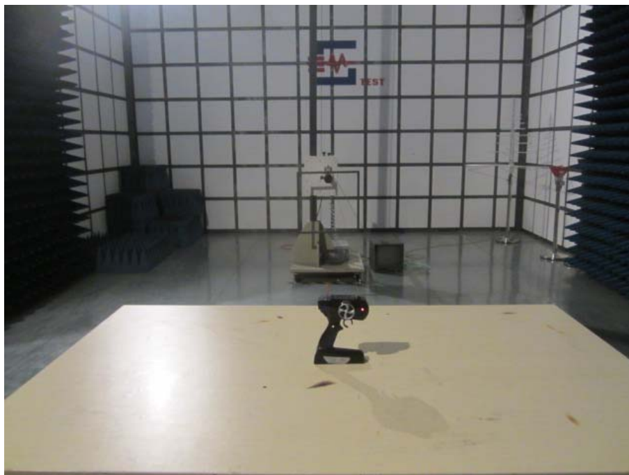
Radiated Emission Test Setup (30MHz to 1GHz)
