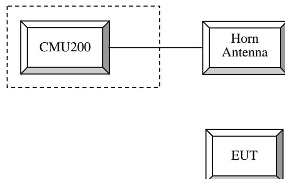
**Block Diagram of Test Setup**
