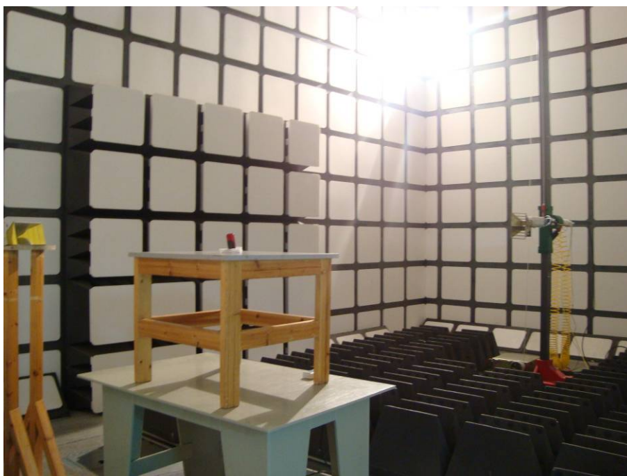
Above 1GHz: Radiated Emissions - Rear View
