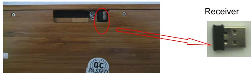
After insert the battery, Please press "Esc" + "Pause Break" simultaneously, low pressure indicator on the right top corner will be light in red, then straight away you put receiver into USB port of PC. The light goes off, there you can start to use.
