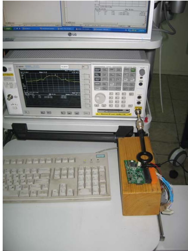
Photograph No.7 Setup for occupied bandwidth measurements
