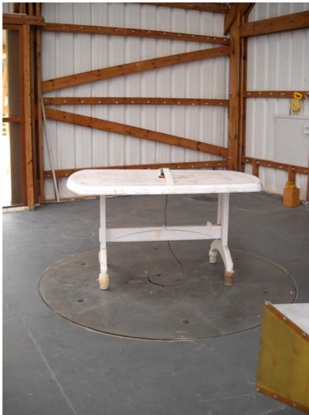
Photograph No.4 Setup for radiated emission measurements at the OATS from 1 to 18 GHz
