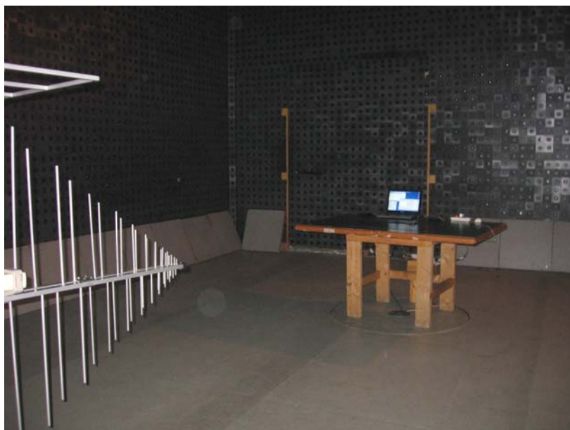
Photograph 7.2.1 Setup for radiated emission measurements in the anechoic chamber
