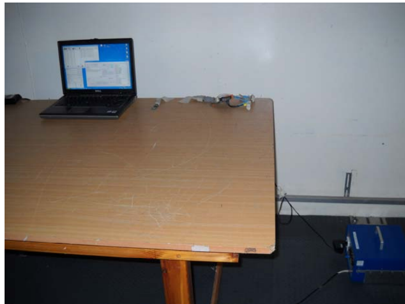
Photograph 7.1.1 Setup for conducted emission measurements
