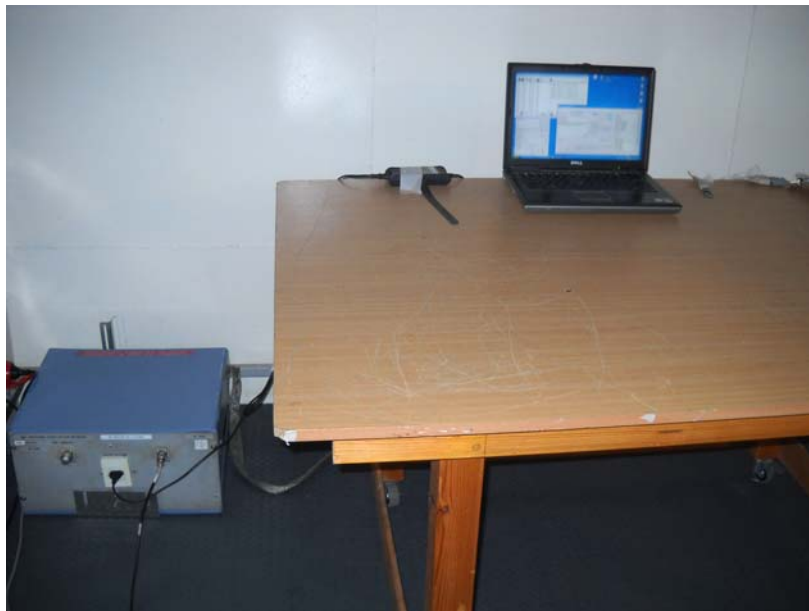
Photograph No.9 Setup for conducted emission measurements on the AC power lines
