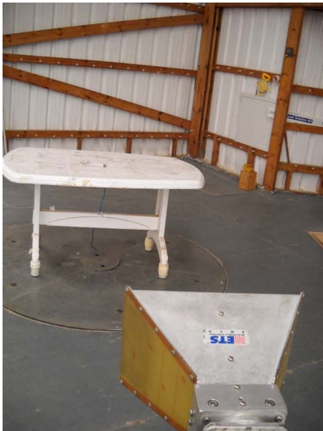
Photograph No.5 Setup for radiated emission measurements at the OATS from 1 to 18 GHz
