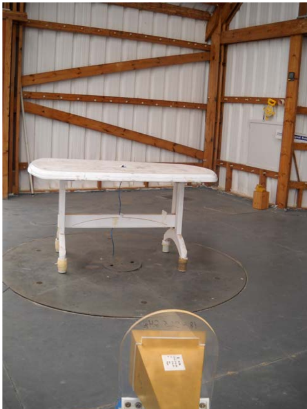
Photograph No.6 Setup for radiated emission measurements at the OATS from 18 to 25 GHz
