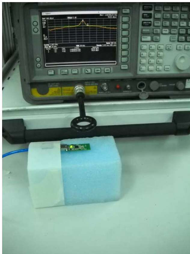
Photograph No.8 Setup for occupied bandwidth measurements
